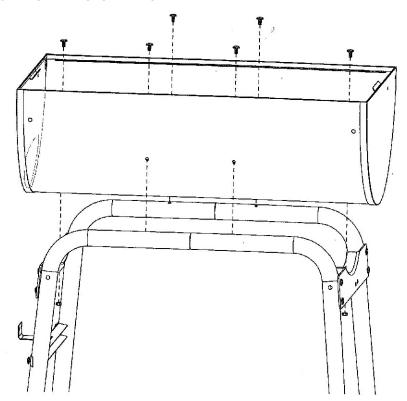
Attach front shelf (item #10) to front of grill base using two M6 x 15mm Phillips head bolts. Attach table supports (item #11) with slotted holes towards front shelf using four M6 x 15mm Phillips head bolts.
